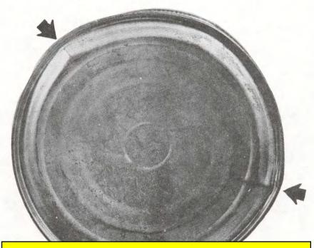
Defect No. 111. Buckle. Major Defect. A permanent distortion of the counter sink (channel next to end seam). Caused by excessive internal pressures developed during processing. The distortion of the end seam is readily noticeable at first glance. There is a some suspicion that the end seam has been placed under tension sufficient to jeopardize the hermetic seal.
