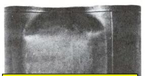
Defect No. 208. Dent. Lower limit of a minor defect. A slight indentation with moderately acute crimping of the body wall resulting in a related minor defect as the end seam is pulled out of position slightly. Must be studied carefully to detect the malposition (minor defect).
