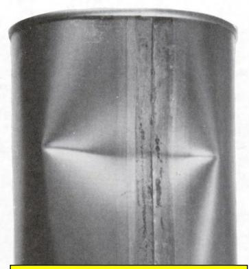
Defect No. 208. Dent. Upper limit of a minor defect. A moderately deep, sharp, angular indentation with moderately acute crimping of the body wall.
