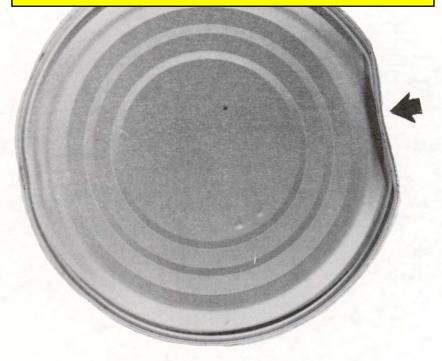
Defect No. 208. Dent. Upper limit of a minor defect. Moderately deep dent on the end seam forcing it inward to such an extent that the counter sink (channel next to end seam) and body are involved, but no sharp ridges are evident.
