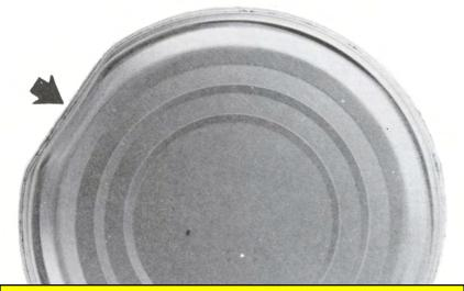
Defect No. 208. Dent. Upper limit of a minor defect. A moderately deep indentation with moderately acute crimping of the end seam.
