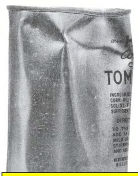
Defect No. 110. Dent. Major defect. A very deep, sharp, angular dent with very acute crimping of the body wall.
