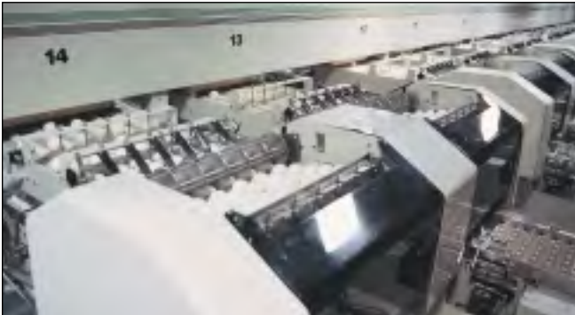
Figure 18. Packaging unit orients eggs with small end down and gently places them into consumer cartons. (99-CS-1608)
