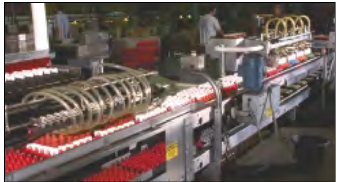
Figure 6. Eggs are automatically transferred from off-line conveyor to conveyor spools going through the egg washer. (CD 8202 3241 1143-31)
