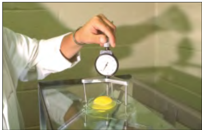
Figure 52. USDA grader demonstrating the use of a Haugh meter by measuring the height of the thick albumen. (CD 8202 3241 1143-17)
