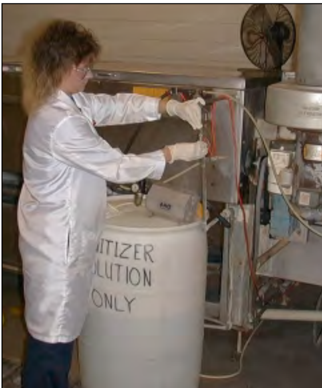
Figure 11. After washing, eggs are sanitized with an approved chemical sanitizer to remove any remaining bacteria. USDA graders verify concentration of sanitizing spray. (00CN0049)
