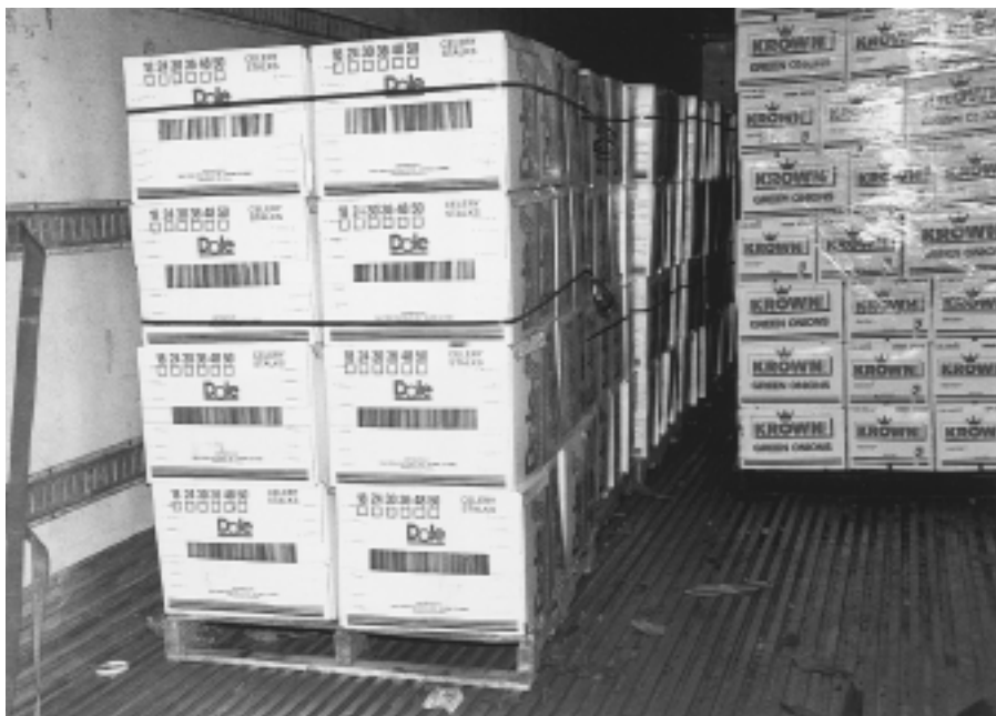
Figure 18. A mixed palletized load of celery and green onions loaded in a unit load airflow pattern.
