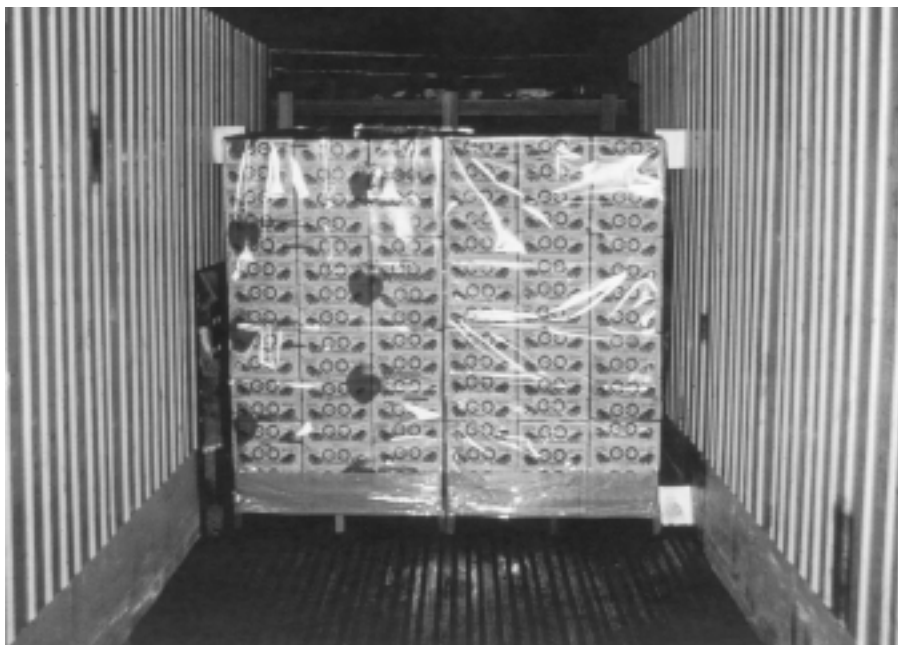
Figure 17. A palletized load of strawberries, center-loaded. (Note: Each pallet load is enclosed in an airtight plastic bag injected with a modified atmosphere.)
