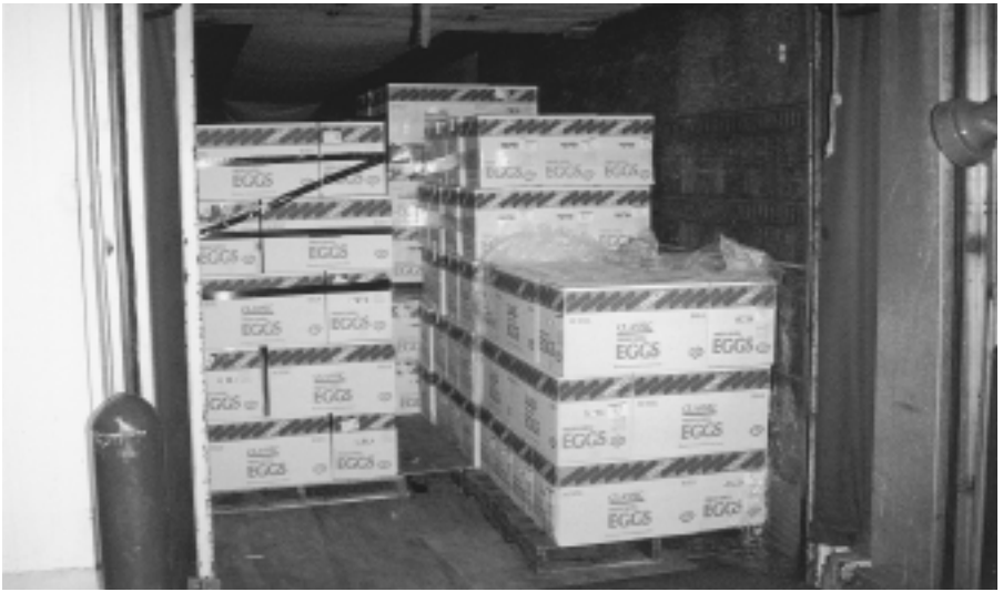
Figure 20. A palletized load of eggs. Note the stretch film around the pallet loads at the rear door area where road shock is greatest.
